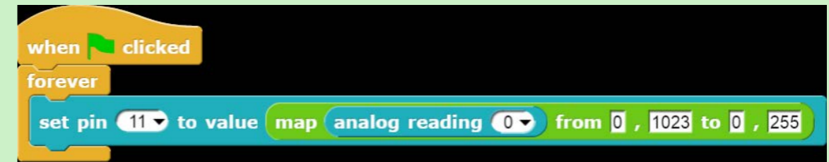
Figure 34. Fade an LED with the potentiometer (you need to import the map block for this program – refer to Lesson 6)
