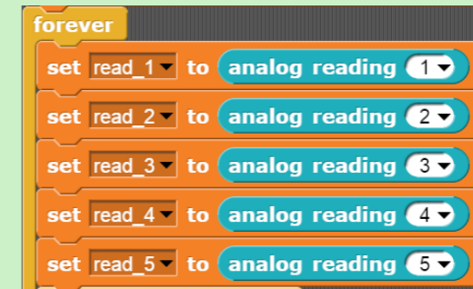
Figure 92. Setting of the read variable at the top of the forever loop
