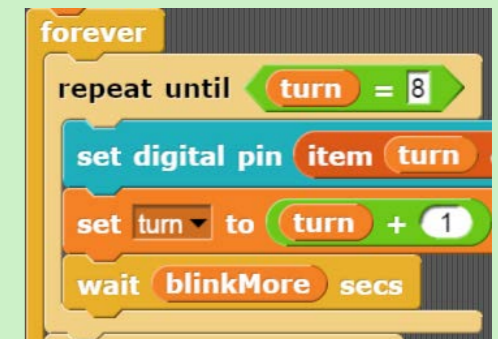
Figure 58. Placing a wait block at the base of the repeat block
