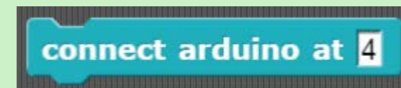
Figure 21. When this block is initiated it will connect the Arduino at COM port 4
