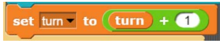
Figure 56. The turn variable used as a counter to add 1 to itself each time
