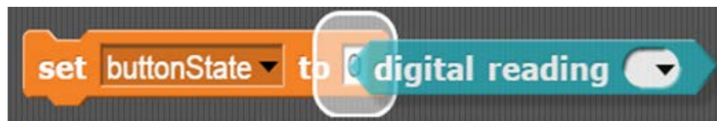
Figure 65. Placing a digital reading block inside a set_to_ block to read the button
