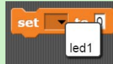
Figure 41. Variable names can be accessed from a dropdown menu on some blocks
