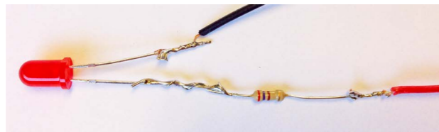
Figure 130. The soldered LEDs with a resistor on one leg
