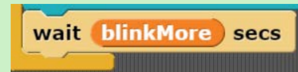
Figure 48. Using the blinkMore variable to set the delay for the wait block
