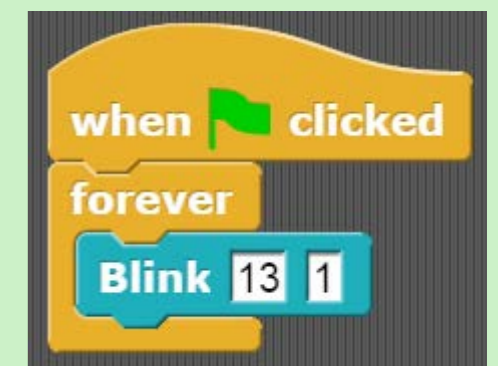
Figure 106. Calling the Blink function within the forever loop with the arguments 13 and 1
