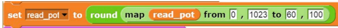
Figure 85. Setting the read_pot variable to a number between 60 and 100 by using the map and round blocks
