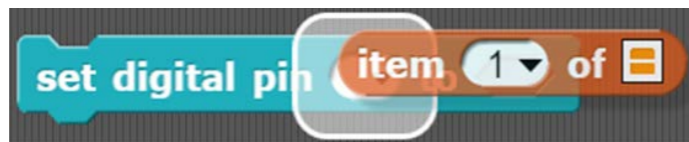
Figure 52. Placing an item_of block inside a set digital pin block
