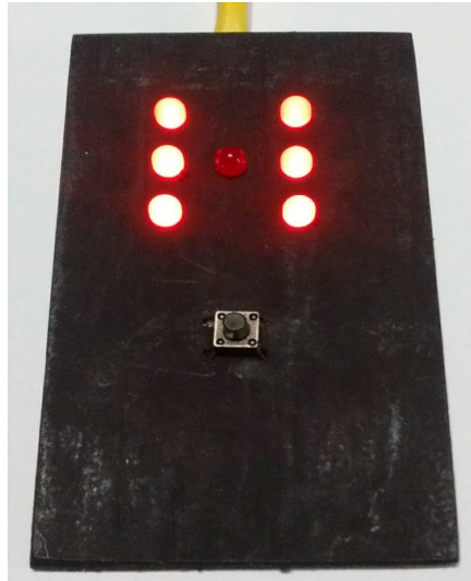
Electronic LED Dice - Switched Activated using 7, long leg, 27 mm long LED's
