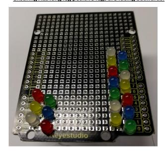
Cover the LED's with masking tape again so you can flip and solder the column 3, positive legs.
