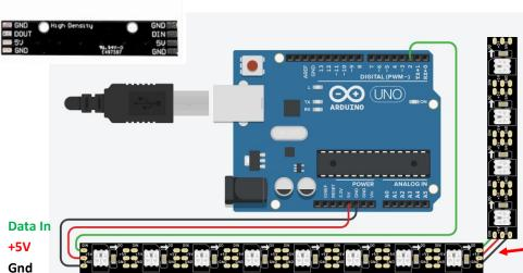
Neo Pixel LED's have a +5V, Gnd and a Data In or DI. They also have a Data Out or DO to connect to another strip, if daisy chaining.
