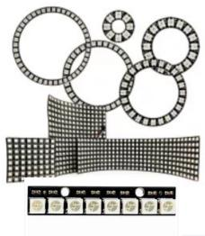
The Neo Pixel (WS2812) RGB LED strip is a strip of LEDs that the colour and brightness of each LED on the strip can be controlled individually. Each LED has its own embedded controllable microchip. They come in rings, sticks, strips, matrices, bendable and more. From just a single pin you can control many LEDs.
