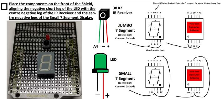
Place a piece of masking tape over the components, so you can flip the shield over for soldering.
