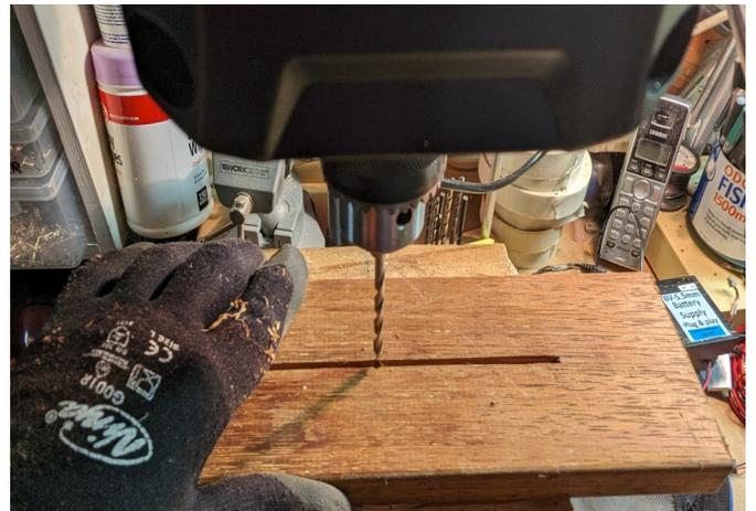
I made up a holding Jig to Rout and enlarge the slots made from the drop saw, from one end .
