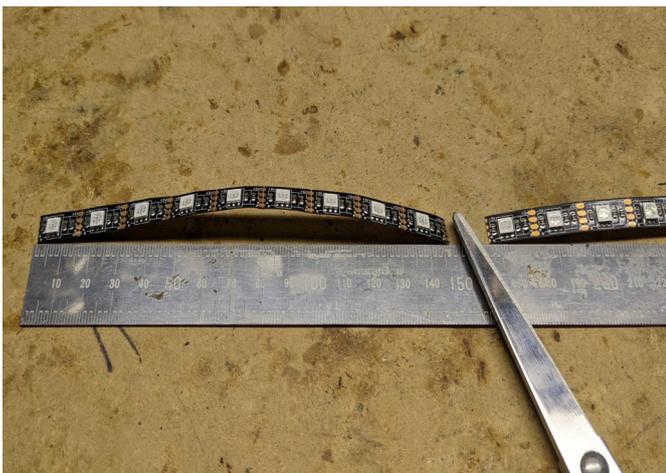
□ Peel off the paper protective strip and stick the LED Strip to a 18mm wide x 150 mm long x 1 mm thick wooden Stirring Stick. ( from the \$2 Craft shop)
