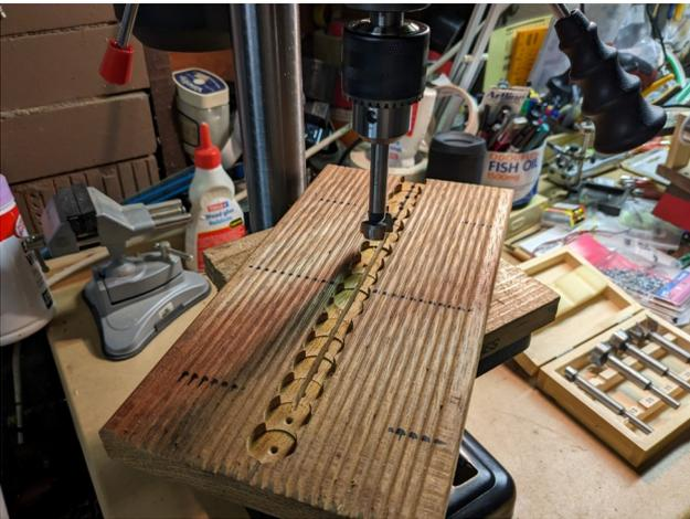
□ Once Routed and sanded, I used a Water Based Satin Cabothane to seal the wood, ensuring not to drop any in the 4mm slot.
