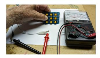
10 — Using a Hot Glue Gun, secure all the wires to the board, to stop them from moving. To stop activating the Makey Makey on the back with your fingers, I secured a clear Acetate Sheet (for wiring identification) or cardboard for insulation, with tape.
