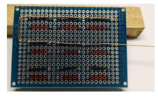
7 — Use a Multimeter and attach it to the Earth (Ground) and to each attached Clip/ Wire to test continuity.
