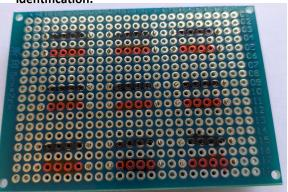
4 — Solder all of the legs to the Prototype Board, to stabilise the switches, when they are pushed.
