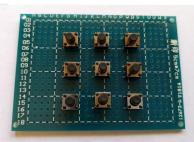
3 — On the back, Draw with a permanent pen, Black (—) and Red (+) lines, between the inserted legs of the switches, for ease of identification.
