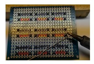
5 — Join and Solder all the Black (—) legs together using Enamelled Copper Wire to form a Ground or Earth to all switches.
