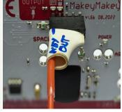
12 — Make up Identification Labels for the Alligator Clip wires for correct connection and connect all wires & Alligator Clips, To the Makey Makey.
