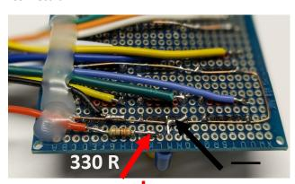
11 — Solder the W,A,S,D wires to a 6 pin Header inserted in the Makey Makey. Attach the (+) wire from the 330 R Resistor to a 5 pin Header inserted in the Makey Makey, to Key Out. Secure with Shrink Tubing if available and label for correct connection.
