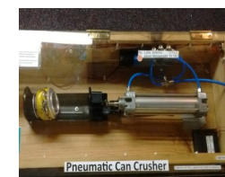
28 - Pneumatic Can Crusher
