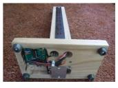
16- Build up Pat's 14 M2 IR Microcontroller & battery. Use Microcontroller and attach in the routed out cavity, to wires through hole in base, using 6mm small self tappers.
