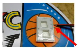
Using a Coping or Jigsaw, carefully cut inside the line.
