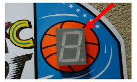
**Carefully Drill inside the 4 corners with 6mm Drill.**
