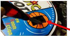
Insert the Jumbo Display from the back, decimal point down.
