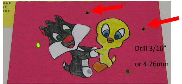
Drill approx. 6mm diameter Hole
