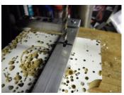
18 – Drill using a 5 mm drill, in 20mm from the end for stage 1 & 5, 50 mm in for stage 2 & 4, 75 mm in for stage 3
