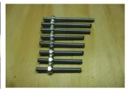
35 - Screw a 3/16 th nyloc lock nut up about 10mm from the bottom.
