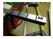
29 –Cut a piece of 30 mm x 30 mm Aluminium Angle to make the hinge brackets.
