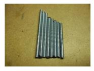
33 - Cut the following for the sloping tracks - 70 mm, 66 mm, 59 mm, 55 mm, 53 mm, 50mm, 49 mm & 45mm. File & debur.
