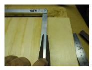
17 – Place the assembled tracks upside and using a pair of dividers scribe the centre lines.
