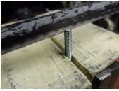
34 - Carefully holding using soft jaws in a vice, centrally, hacksaw blade cut a groove slot approx. 2 mm deep on one end only.
