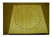
9 – Cut a 12mm thick, piece of 5 ply, 250 mm x 250 mm base, sand & seal. Scribe a 100 mm radius, drill 5 mm top,6 mm bottom holes for LED's at 18 mm centres.
