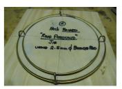
8 – Solder at 90 degrees spacings, joining the Inner & Outer Rings. This will give ~ 12 mm gap for the ~16mm diameter marbles.
