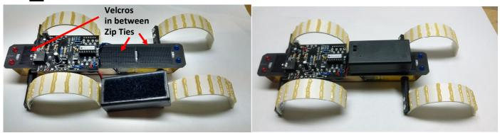
Build Pat's 14M2 Motor Driver Microcontroller, attach to the Top Plate with velcros or double sided tape.
