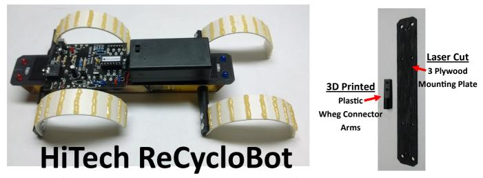
Below are some of the Production Steps, or you can use your own design. Tick off each box as you complete a task and Document it. Tools Required - Soldering Iron, Pop Rivet Gun, Small Zip Ties, Small Phillips Head Screwdriver, Hot Glue Gun, Drills, Velcro Tape.
