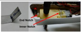
IMPORTANT – Zip Tie Motors to top plate & Align carefully, centrally & 15mm in from ends. Then push on assembled Wheg Connector Arms.
