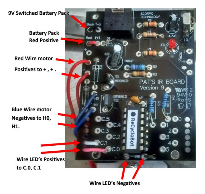
Note - If the Motors/Whegs are going in different directions, swap the Positive and Negative wires around on one motor only, at the motor.
