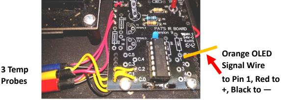
**How to Connect to your 14 M2 Mi-Battery Pack Black Negative Battery Pack Red Positive Red OLED wire** Positive to (+) 3 Red Probe wires to Version 9 Positive (+) **Orange OLED Signal Wire** to Pin 1 3 Temp **Probes Black OLED wire** 3 Black Probe wires to Negative to (— ) Negative (-)
