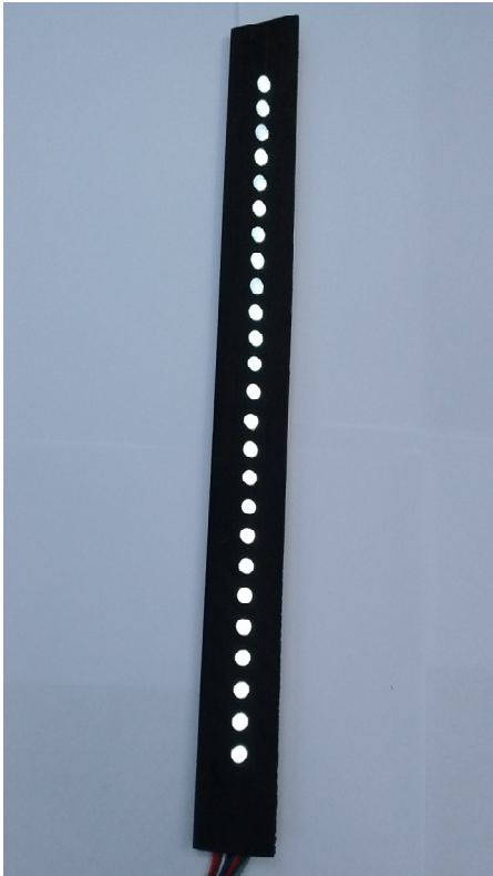
25 White LED’s on 300 x 30 x 3 mm Plywood Strip
