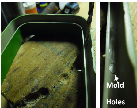
4- With the frame face down, carefully drill (4.8mm drill for the 5mm LED's) the 20 holes for the LED's, accurately using the mold holes as centres, taking care not to crack the frame.
